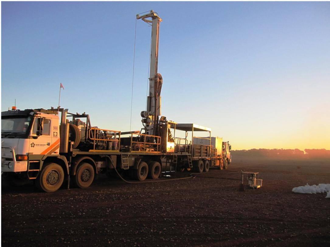
**Figure 1, Sonic Drill Rig (Boart Longyear) on Dynasty's Prairie Downs Iron Ore Project**
