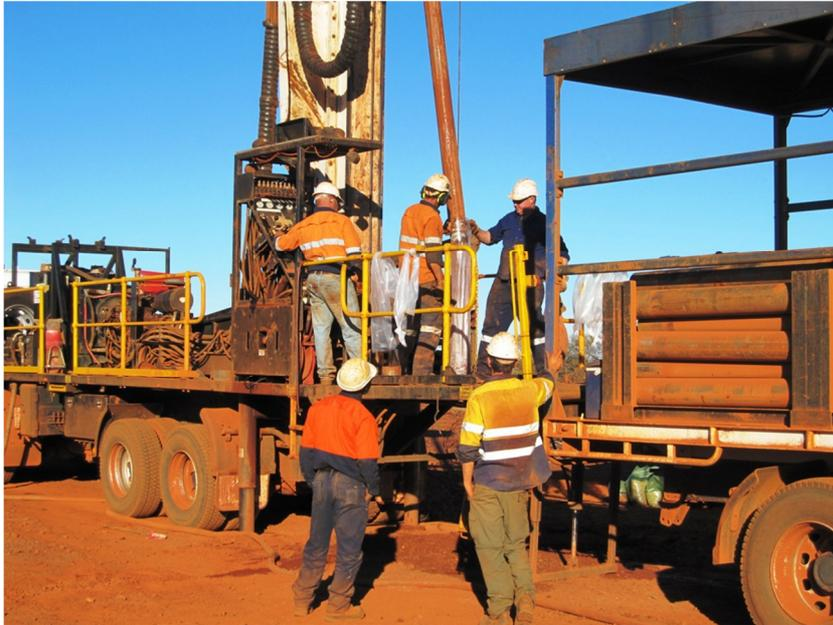
**Figure 3 – collecting a sonic drill sample**
