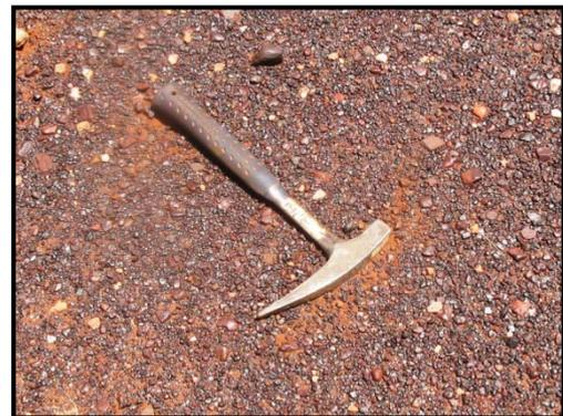
**Plate 1** - showing surface of detrital deposit, relatively even grain size distribution of in-situ material
